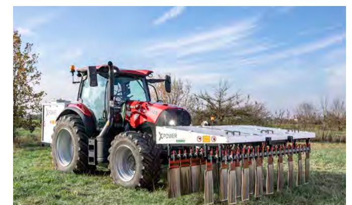
XPower electro-herbicide for zero-chemical weed control
