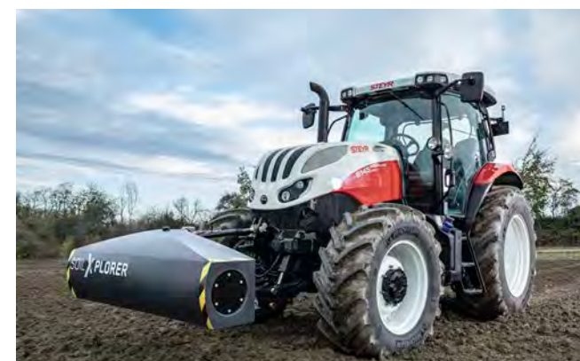
SoilXplorer, the real-time soil scanning system
