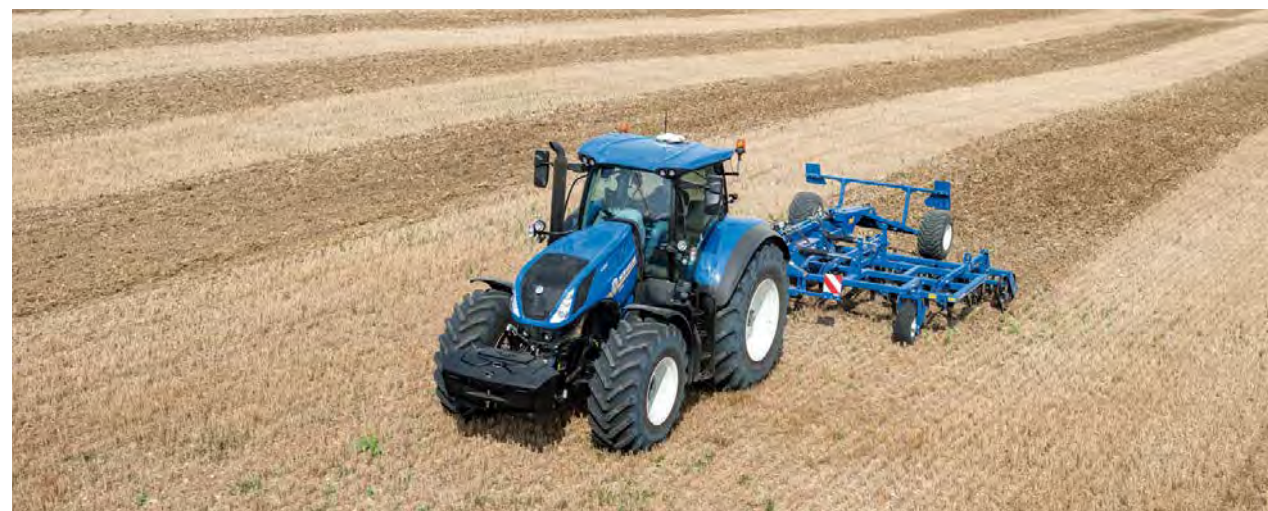
New Holland T7.315 Tractor with Auto Command™ continuously variable transmission
