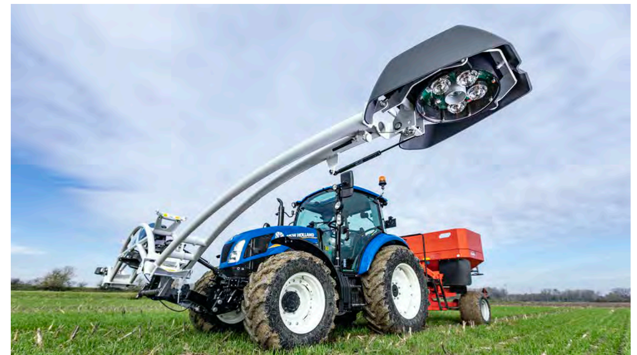
CropXplorer sensor for optimized nitrogen balance
